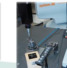
CMM in-process dimensional verification plus final dimension certification to ADP-MI gaging ball datums are possible
