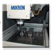
Manual inspection utilizing engineered Programming datum ADP-MI gaging ball datums
