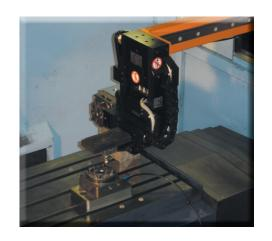
Manufacturing: All components to be machined that are mounted on pallets and programmed to the ADP-MI Precision Gage Ball, can be machined in a variety of CNC machines, as long they are system 3R® Macro pallet receiver-equipped. After machining, they can be verified to file dimensions generated in reference to the gage ball.
